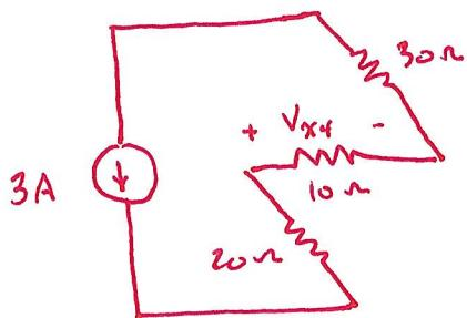
$$V_{x4} = (10\text{ }\Omega)(3\text{ A}) = 30\text{ V}$$
