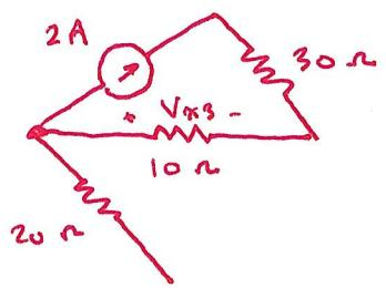
$$V_{x3} = -(10\text{ }\Omega)(2\text{ A}) = -20\text{ V}$$
